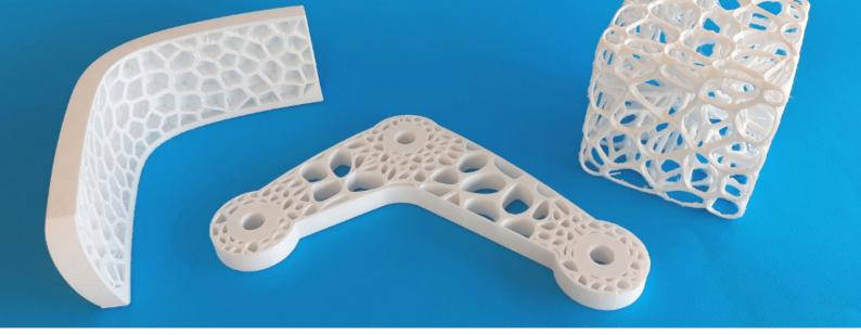
Topology optimisation presents a radically different method that does not rely on predefined design choices but focusses instead on optimising a performance criterion and considering all possible designs that meet the physical and geometrical constraints. By adapting the material distribution on a fine mesh over successive FEM simulations, the best designs that maximise stiffness, minimise weight or reduce vibrations are found.
